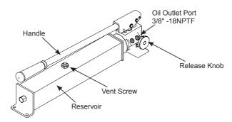
Figure 2 - Model P2001-5K Components
